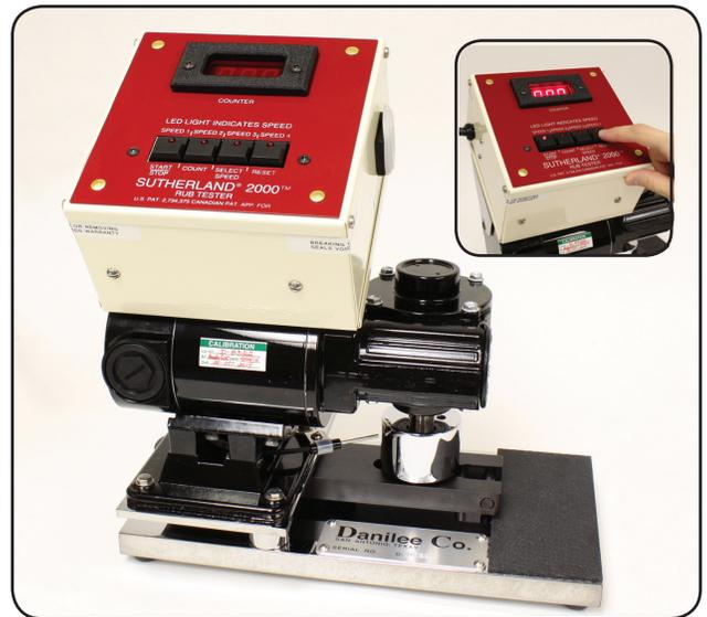
▲ Sutherland Rub Tester showing two pound and four pound weights and the scoring device. The upper receptacle of the timer is for remote timer control. The lower receptacle is the same voltage as the instrument. !
