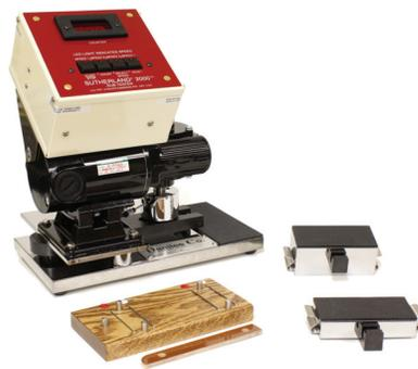
The Sutherland Rub Tester is designed to evaluate the scuffing or rubbing resistance of the printed or coated surface of paper, paperboard, film, etc. The test results are reproducible.
