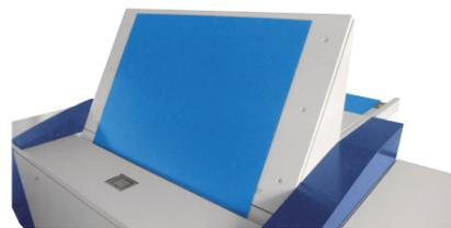
In addition, if the next new plate is set on set table during exposure, the next new plate is loaded automatically just after exposed plate is discharged to the processor.
