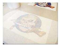
6) Apply application tape over complete image without tiling or creating a seam. For small text (under .75") weed and apply application tape within one hour of cutting. Some curl might occur after one hour due to the thin T-Printz™.
