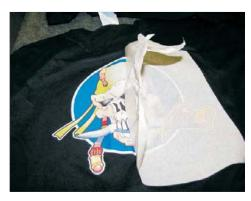
11) After cooling peel back release liner at a sharp angle.
