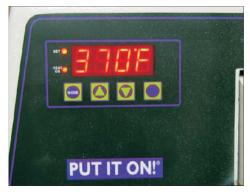
3) Set temperature on press to  $370^{\circ}$  -  $375^{\circ}$ F or  $188^{\circ}$ C -  $190^{\circ}$ C ( $100^{\circ}$ C Cotton)
