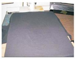
7) Press fabric only for 5-10 seconds to remove any moisture from shirt or fabric.
